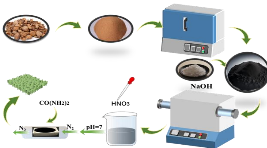
Fig. 1: Schematic of the synthesis procedure of NWSC x ( x = 0.4, 0.5, 0.6 and 0.7 ).
